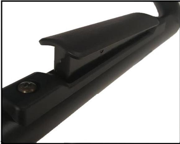
This product was specifically designed for off-highway vehicle applications including agricultural and construction equipment that requires a remote inside release. The robust construction is incorporated into round tubing with 90 degree ends for ease of mounting onto a flat door panel. It also provides support for the opening and closing functions of the door and greater ease of operation (ergonomics) over direct releases.
